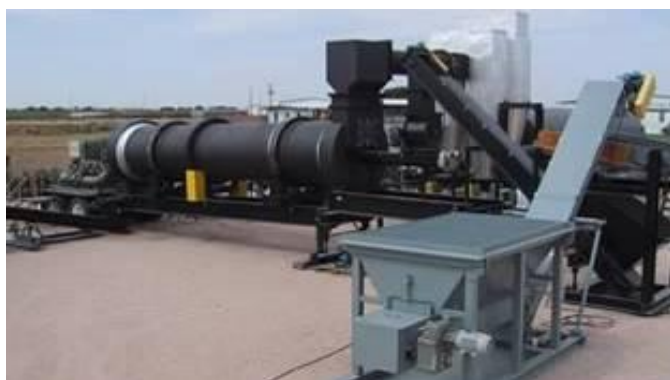
MRC2 mobile Rotary incinerator
