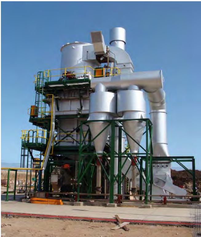
RC2 Pollution control system & secondary phase high temperature Combustion system
