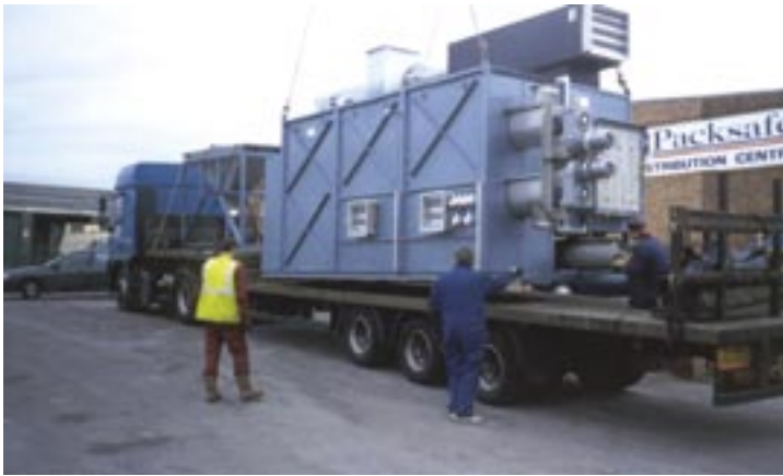
TD5000 Mobile Thermal Sludge treatment system 0.5 to 1m 3 / hr
