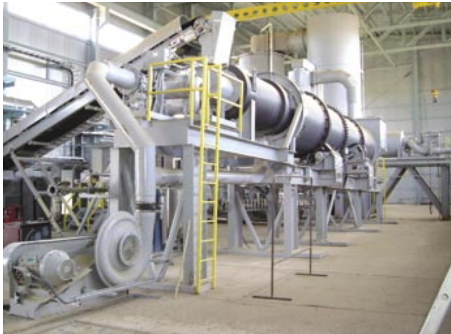
Model RC2 Thermal treatment system for Oil Based Drill cuttings - Middle East
