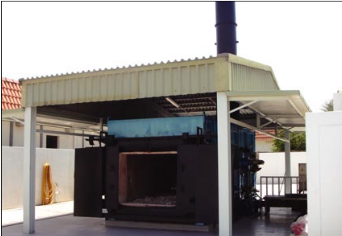
PD288 Oil Fired Incinerator capable of 500 kg/hr throughput
