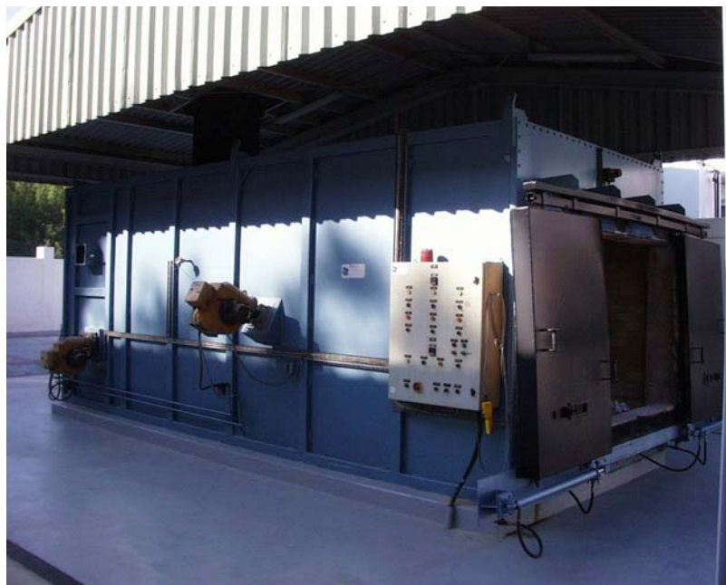
PD288 Animal Carcass Incinerator - Throughput 500 Kg per hour
