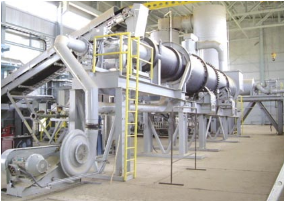
RC500 Oil Fired Incinerator capable of 1500 kg/hr throughput
